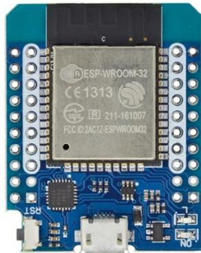
Here is the pinout of the board, if you look at this you can see that the white rows are the same as the Wemos Mini, this means if you fit a suitable header you can use those shields
