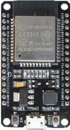
The ESP32 development board, such as the ESP32 DEVKIT DOIT, is based on the ESP32 microcontroller and has both Wi-Fi and Bluetooth functionality. The development board operates at 3.3 V and is powered through a micro-USB connection at 5 V or directly on the 3.3V *VIN* pin, but the former connection is recommended. The GPIO pins are not 5 V tolerant, and the maximum current supply from a pin is 12 mA.
