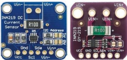
Both current and voltage are measured with the INA219 module, which has at least two formats, from which the corresponding power and energy over time are derived. The *Adafruit INA219* library instructions
