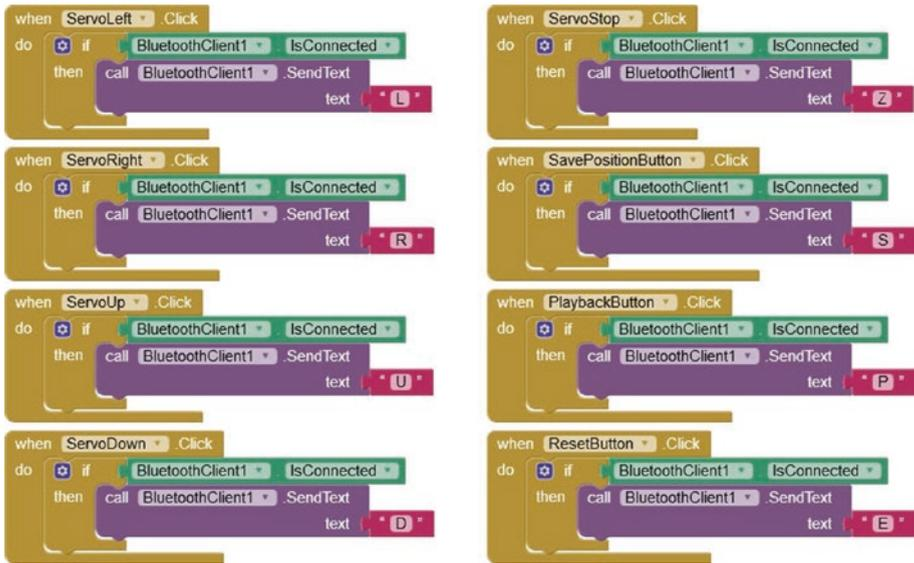
**Figure 10-14.** Servo motor commands
