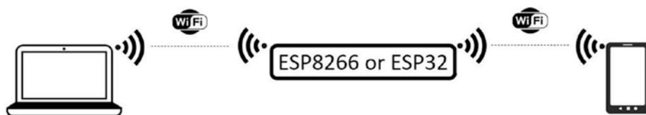
**Figure 7-1.** *Wireless local area network with the ESP8266 or ESP32 microcontroller*
