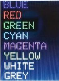
The 2.4-inch ILI9341 SPI TFT LCD touch screen with 240 × 320 pixels has touch screen functionality for displaying text and drawing shapes with different colors on the screen. The acronyms SPI, TFT, and LCD represent Serial Peripheral Interface, Thin-Film Transistor, and Liquid Crystal Display, respectively. The ILI9341 SPI TFT LCD screen and the ESP8266 and ESP32 microcontrollers
