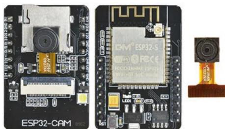
The ESP32-CAM module is based on the ESP32-S microcontroller and includes a 2M-pixel OV2640 camera and a micro-SD (Secure Digital) card slot. JPEG files of images are stored on the micro-SD card or loaded to a
