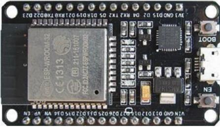
The ESP32 microcontroller includes two 8-bit DACs referenced as DAC1 and DAC2 on GPIO 25 and GPIO 26. The instruction `dacWrite(DACpin, value)` generates a voltage of  $value \times VCC/2^8$ , where  $VCC$  is the operating voltage of the ESP32
