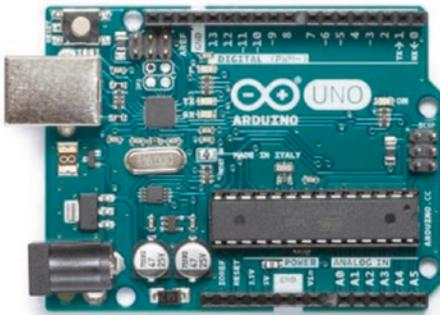
The Arduino Uno is based on the ATmega328P microcontroller, and the development board operates at 5 V, powered through a USB connection at 5 V or a DC input jack at 7–12 V. The maximum current supply from a GPIO pin is 40 mA, with a maximum current from all output pins of 200 mA. In a sketch,
