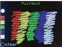
The sketch in Listing 3-5 draws images on the ILI9341 SPI TFT LCD screen when the screen is pressed with a screen pen, with colors selected from a color palette. The first section of the sketch installs libraries and defines the touch screen pins and the paintbrush size. The *setup* function sets the
