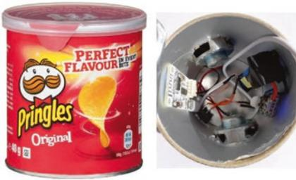
The 18650 lithium-ion battery and T6845 USB lithium-ion battery charge and boost converter module, the Bluetooth stereo audio receiver module with the PAM8403 class-D audio amplifier, and the speakers are easily incorporated in a cylindrical container, such as a 40 g
