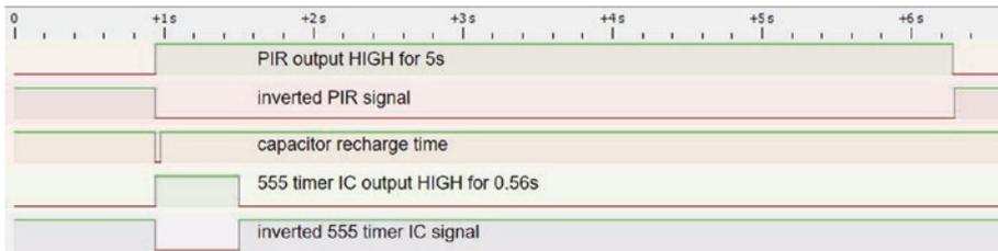
**Figure 17-25.** PIR sensor and MP3 player signal sequence
