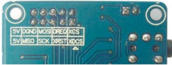
**Figure 1-2.** VS1053 connections
