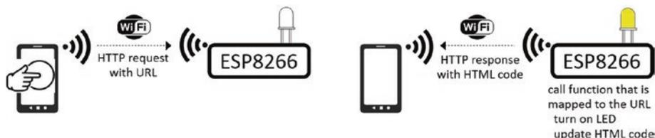
**Figure 7-4.** Client HTTP request and server HTTP response
