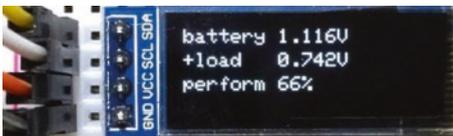
A battery is measured with and without a load using a bipolar junction transistor (BJT) 2N2222 to turn on or off the battery current to a load, consisting of a low-value
